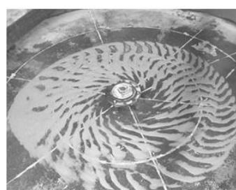
(ب)  $Q_i=0.9 \text{ L/s}$ ,  $D=44 \text{ cm}$ ,  $L_1=41.5 \text{ cm}$
